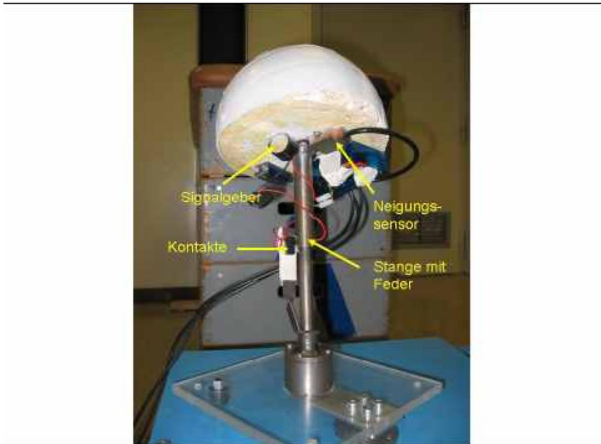
Figure 9: Set-up of the sensor
