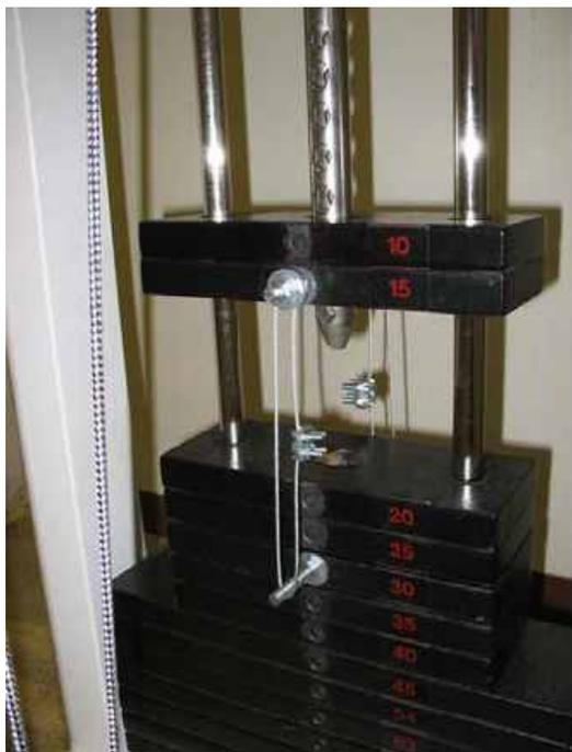
Figure 12: Mechanism with loops for adding weights
