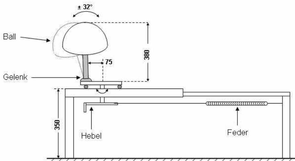
Figure 8: Schematic representation of the ball test
